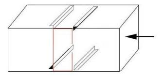
Slide the heat exchanger carefully into the plenum to check the fit again. Once proper fitting is verified, you can seal off the ends of the heat exchanger and the hole you made in the plenum with foil or duct tape.
