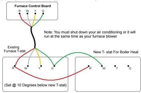
Use the example drawing below if you have a 2 wire system or the thermostat is the advanced computerized type that communicates back and forth between the furnace (typically found on heat pump systems). **Do not use this method if your HVAC system utilizes a multi-speed blower.** All of the parts below are available through your dealer or Nature's Comfort.
