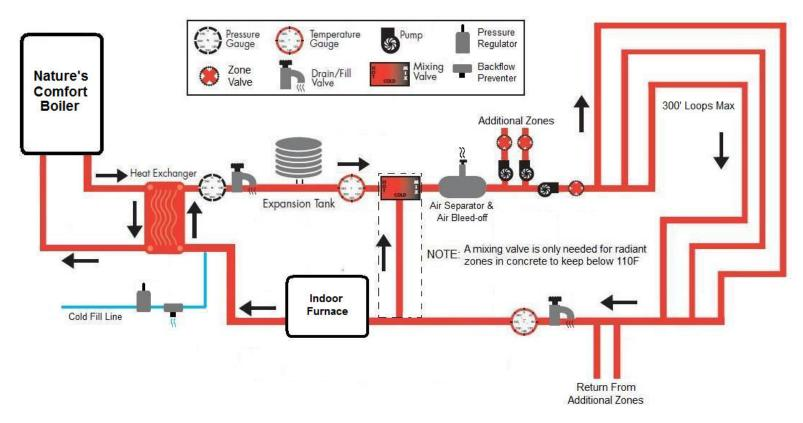
As shown in the above figure, the two systems are totally isolated from each other so that the existing hydronic system remains undisturbed and functions exactly as it did before. Water that circulates through the outdoor boiler is never circulated through the home's hydronic system or vice-versa.
