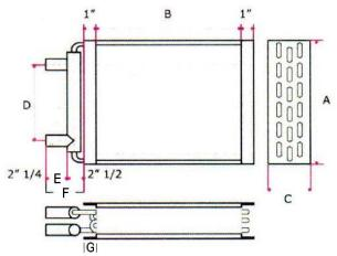
Start by cutting a hole in the side of the ductwork the thickness of the heat exchanger (Dimension C) and the full length of the ductwork (usually Dimension A).
