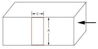
Cross section of plenum showing air blowing in it from right cut hole where red lines are.
