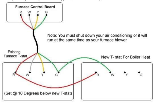
Use the example drawing below if you have a 2 wire system, don't have a blower-only function or the thermostat is the advanced computerized type that communicates back and forth between the furnace (typically found on heat pump systems). **Do not use this method if your HVAC system utilizes a multi-speed blower.** All of the parts below are available through Nature's Comfort.
