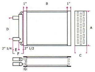
Start by cutting a hole in the side of the ductwork the thickness of the heat exchanger (Dimension C) and the full length of the ductwork (usually Dimension A).
