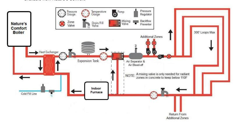
As shown in the previous drawing, the two systems are totally isolated from each other so that the existing hydronic system remains undisturbed and functions exactly as it did before. Water that circulates through the outdoor boiler is never circulated through the home's hydronic system or vice-versa.
