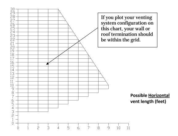
Let's imagine an installation consisting of a 4-feet vertical rise, a 90-degree elbow, followed by a 7-feet horizontal run through the wall, ending with a termination cap. This type installation is not acceptable. As you can see, the vent termination is clearly outside the allowed configuration zone on the chart. The venting system does not have at least one foot of vertical rise for each foot of horizontal run. Furthermore, it does not have a minimum elevation of 3 feet on the outside wall.
