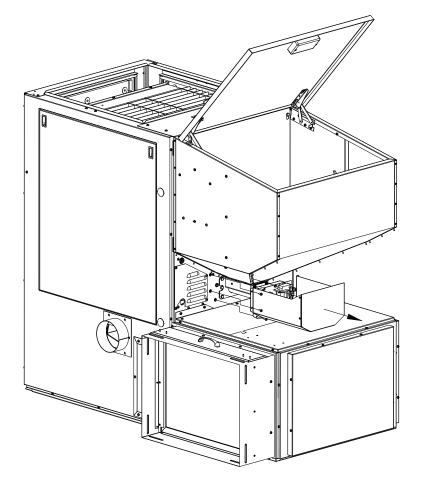
2- Remove the screws from the hopper support (keep the screws).
