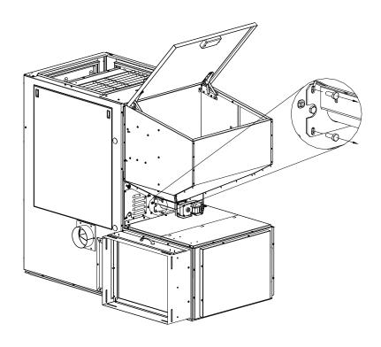
3- Loosen the screws inside the hopper. Lift it and pull it backwards.
