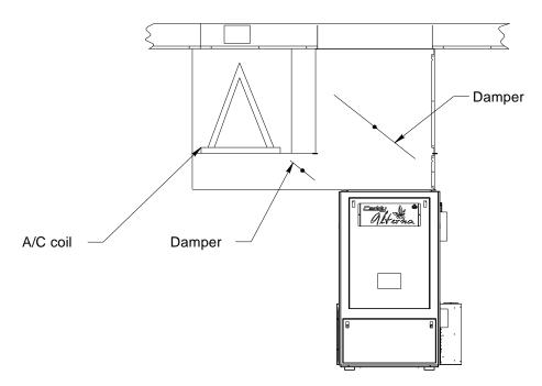
Recommended Installation with an AC unit
