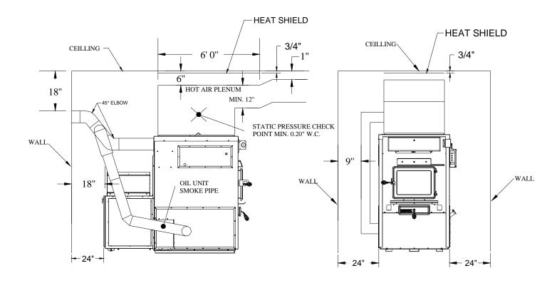
N.B. FOR THE AIR RETURN, RESPECT THE OPENING SURFACE OF THE COLD AIR PLENUM OF THE FURNACE.
