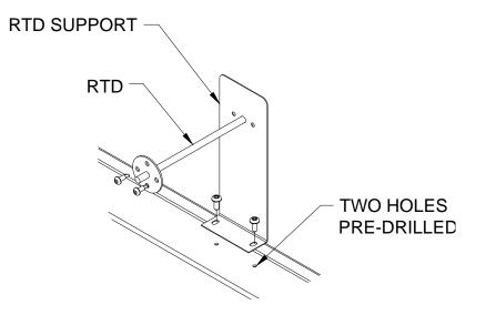
It is important that the RTD and the RTD support be properly fixed onto the ducting system.
